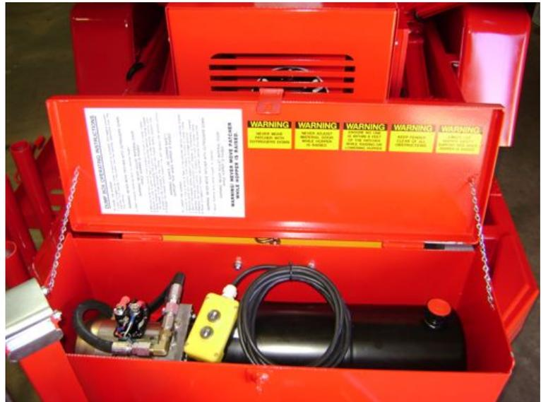
**WARNING: ALWAYS USE THE CYLINDER GUARD (STORED ON HINGED SIDE OF TOOLBOX) WHEN THE HOPPER IS IN THE RAISED POSITION AND REMOVE/REPLACE BEFORE LOWERING.**
