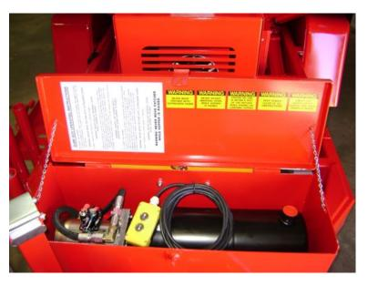
WARNING: <u>ALWAYS USE THE CYLINDER GUARD (STORED ON HINGED SIDE OF TOOLBOX) WHEN THE HOPPER IS IN THE RAISED POSITION AND REMOVE/REPLACE BEFORE LOWERING.</u>
