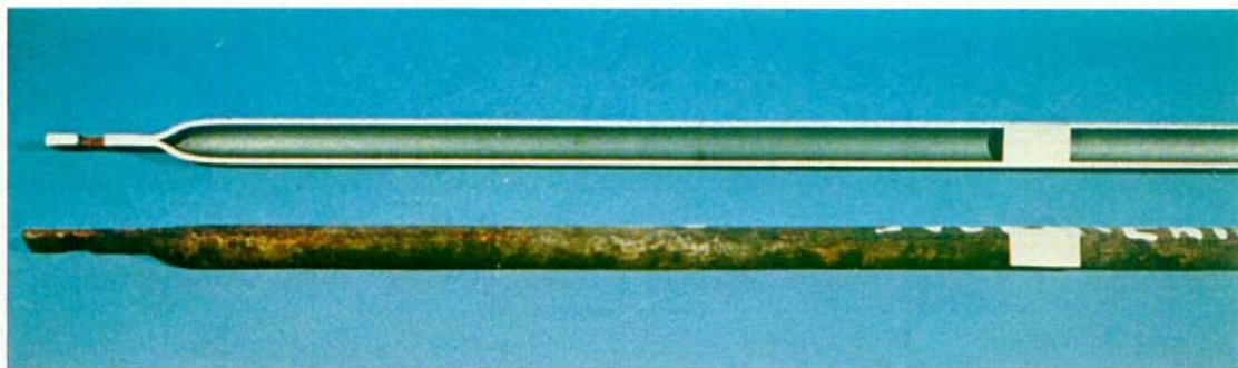
Figure 57: Flattened end tube (First inspection programme)
