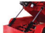
Dump System - Pivot Point & V-Body
